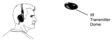
Using the headphones with your system allows rear-seat passengers to listen to their DVD or video game without disturbing front-seat passengers. When using the headphones the IR transmitter dome must have a direct line of sight to the headphones to work properly.
